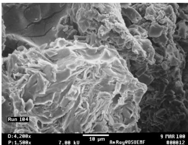
Figure 3. SEM photomicrograph of itraconazole formed at the treatment condition: with SC CO 2 (P=300 atm), T=135°C and t=10 minutes.
